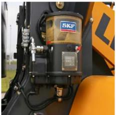
An optional, automatic greasing system improves bearing life and reduces repairs by delivering regular and precise amounts of grease to each bearing.
